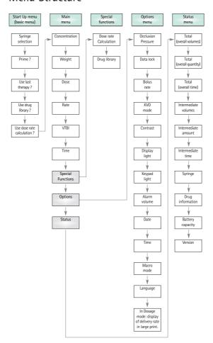
The pump can be customized to the user's needs by deactivating the functions of the start-up and option menus as well as the bolus function via the service program.
